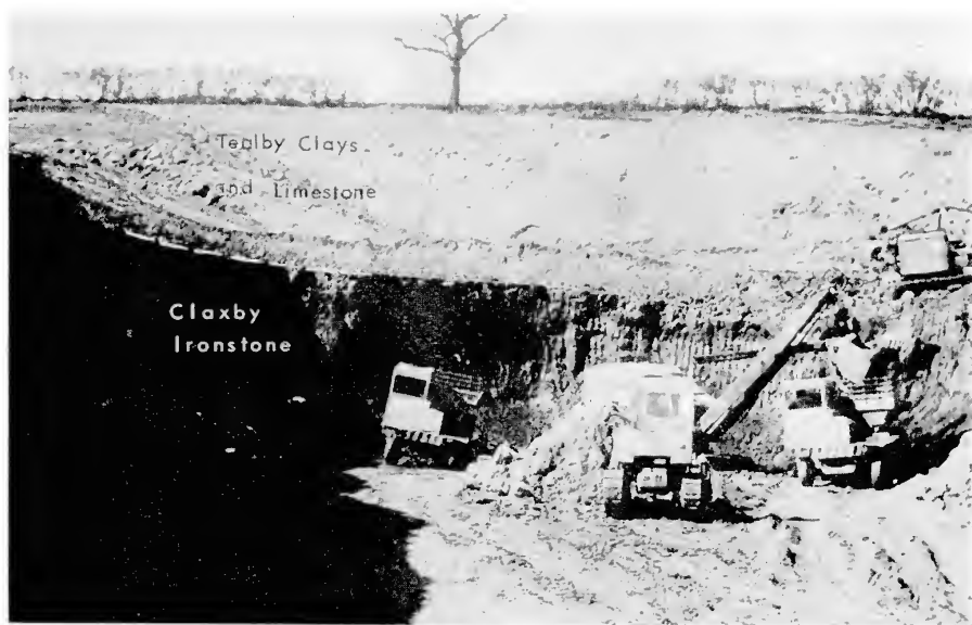
Plate 7. Former open-cast working for Claxby Ironstone (overlain by Tealby Clays and Limestone) at Nettleton. (TF 120978)
